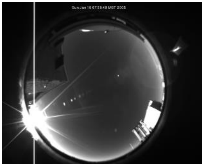
Figure 6: StellaCam image taken just after sunrise. In this image the StellaCam was configured to run at full video rate with the gain set to the minimum value. The automatic iris is running here; otherwise, the entire image would be saturated.
