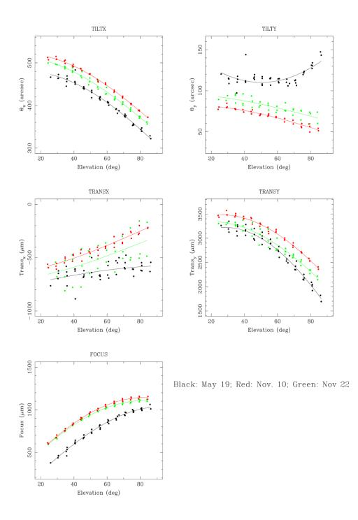
Figure 1: Results from the WFS data taken to calibrate M2 open loop corrections. The data in black were taken before summer shutdown on May 19. The red and green data are post-shutdown from the nights of November 10 (red) and November 22.
